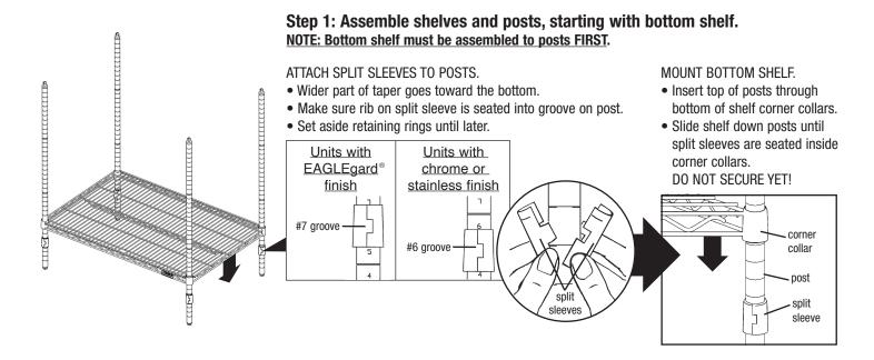
**IMPORTANT**: IF YOU HAVE OPTIONAL CENTER SHELVES, THEY MUST BE INSTALLED IMMEDIATELY AFTER INSTALLING BOTTOM SHELF. REPEAT STEP 1 TO MOUNT OPTIONAL CENTER SHELVES (IF ANY), WORKING FROM BOTTOM TO TOP.
